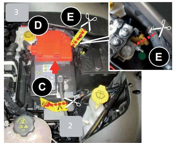
NUR DAS KABEL ENTLANG DES ETIKETTS DURCHTRENNEN, ODER AUF JEDEN FALL AM AUSGANG DES STECKERS
